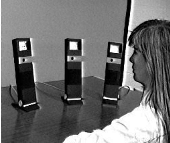
Figure 3. A four-way videoconference using Hydra. Each Hydra unit contains a video monitor, camera, and loudspeaker. A single microphone conveys audio to the remote participants.
