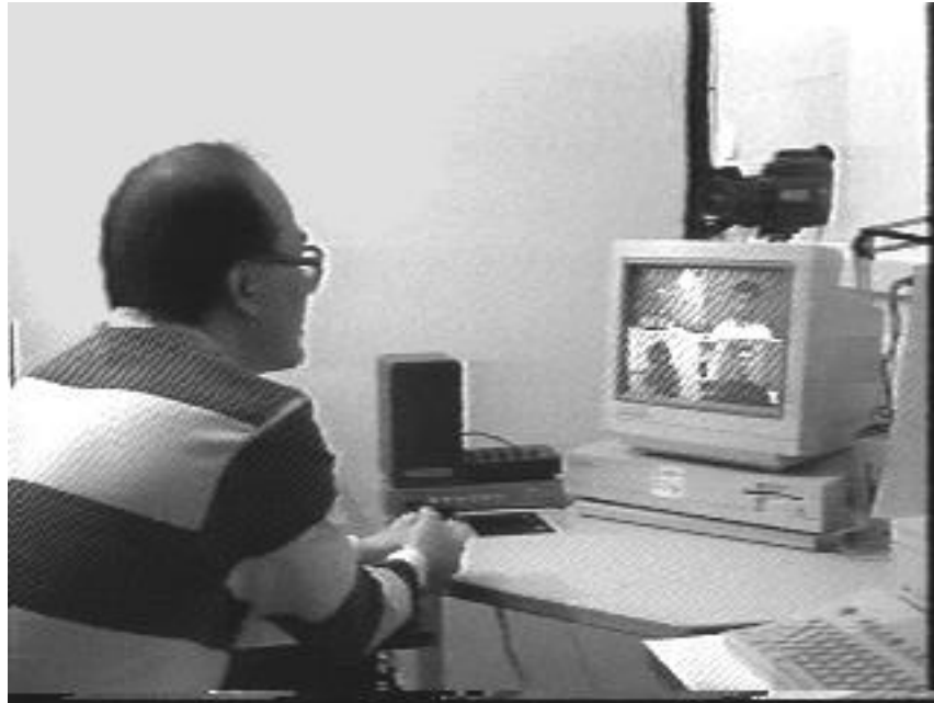
Figure 2. A four-way videoconference using a PIP device. All participants see the same split screen, which includes an image of themselves.
