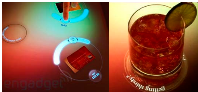
Figure 1.2.5: Recognizing a Credit Card and a Drink on the Surface. Objects can be identified by techniques such as shape recognition, or tagging using approaches such as optical bar codes or RFID tags. Based on context, the surface can then enable certain relevant transactions. Microsoft (2007) [9].
