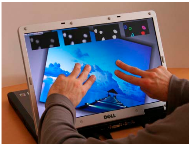
Figure 1.2.9: ThinSight: An Integrated Optical Multi-Touch- Sensing Thin-Form-Factor Display (Hodges, et al., 2007 [6]). The fingers are illuminated by IR from behind the LCD, and the fingers are detected by the IR light reflected back through the display. The black background rectangles show the finger shadows.
