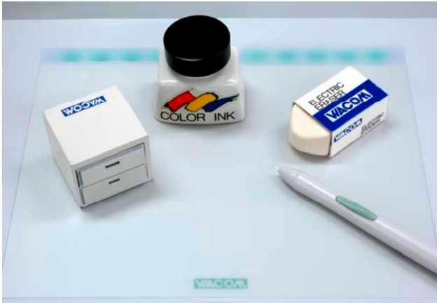
Figure 1.2.7: The Wacom Paint Phycons (Fukuzaki, 1993) [4]. The physical icons can be seen on the graphical tablet: the filing cabinet, ink-pot, eraser, and stylus. The system worked using electro-magnetic resonance. Each phycon had a coil in it with a unique resonant frequency, determined by its unique coil length. Hence, each device could be identified, as well as location determined, by the tablet circuitry. No batteries or wires to the devices were required. (Photo compliments of Wacom).
