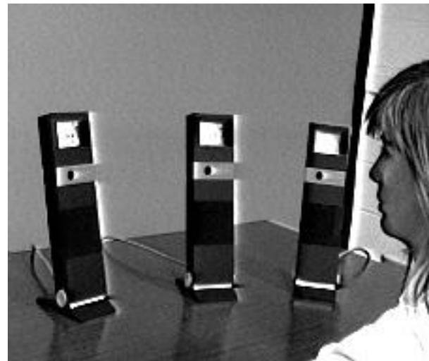
Figure 4: A user is seated in front of three Hydra units. In the photo, the Hydra units sit on the table in the positions that would otherwise be occupied by three remote participants. Each Hydra unit contains a video monitor, camera, and loudspeaker. A single microphone conveys audio to the remote participants (From Buxton & Sellen, 1991).
