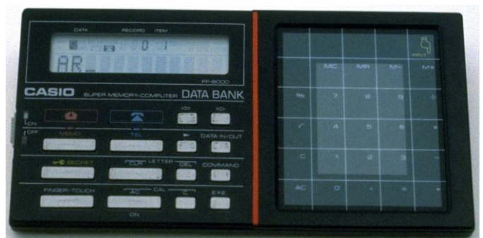
Figure 2: The PF-8000 Data Bank (1984). Characters can be entered by printing them on the touchpad with a finger.
