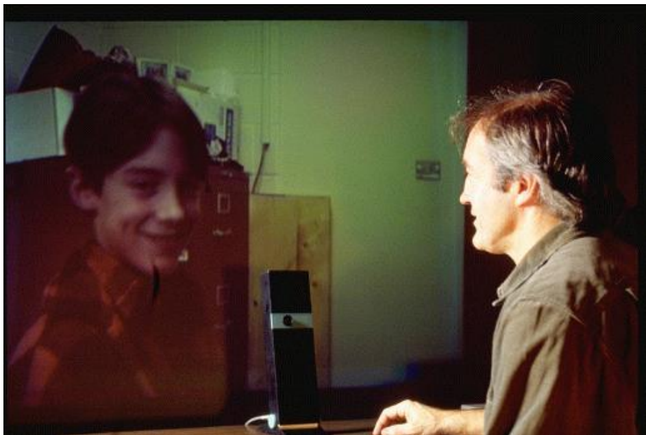
Fig. 13.7 Face-to-Face. In this scenario, each participant has a computerized desktop on which the same information is displayed. The intention is to capture the essence of working across the desk from one-another. Each sees the remote participant life-size. The video camera (from a Hydra unit) is unobtrusive on the desk. Participants interact with the computer using a stylus. When one participant looks down to their desktop, their eyes seem to project into the space of the other, thereby strengthening the sense of telepresence. While there is a considerable amount of technology involved, it is integrated into the architectural ecology. What one gets is lots of service and lots of space, not lots of gear and appliances.
