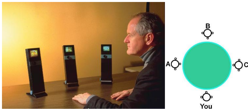
Fig. 13.5 Using Video "Surrogates". The photo on the left shows a 4-way video conference where each of the three remote participants attends via a video "surrogate." By preserving the "round-table" relationships illustrated schematically on the right, conversational acts found in face-to-face meetings, such as gaze awareness, head turning, etc. are preserved.
